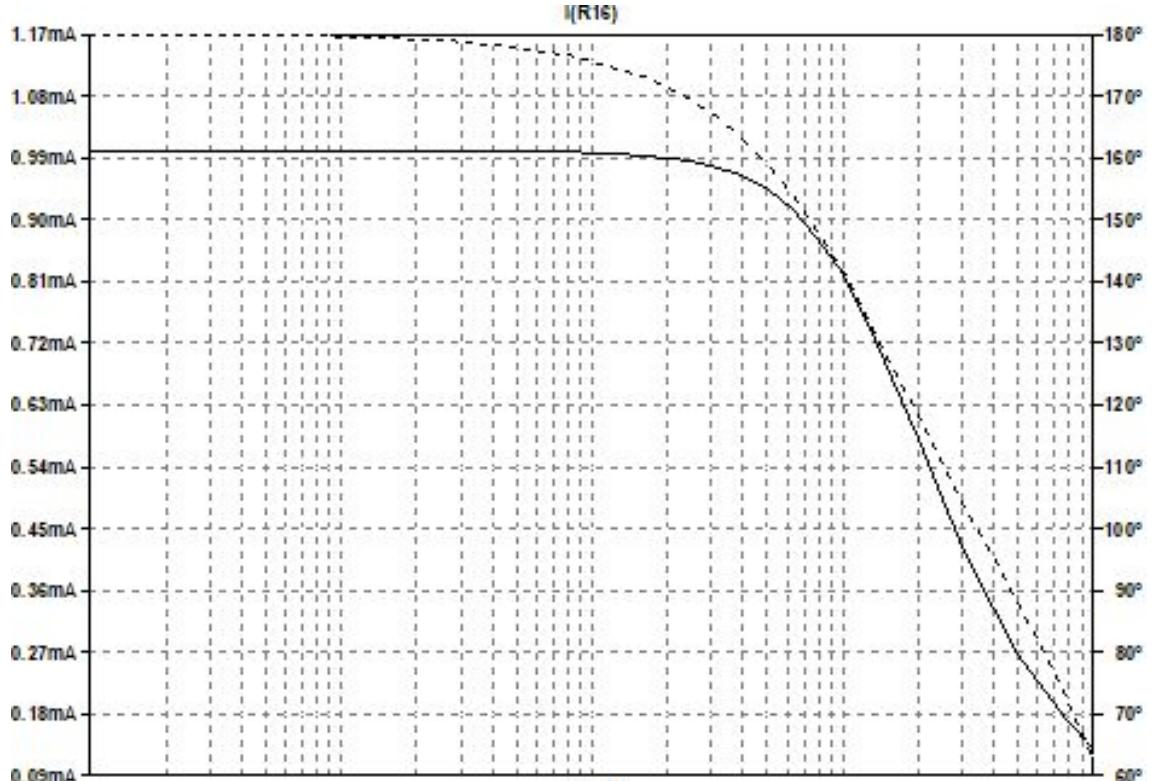
Load =  $1\text{ k}\Omega // 1\text{ nF}$
